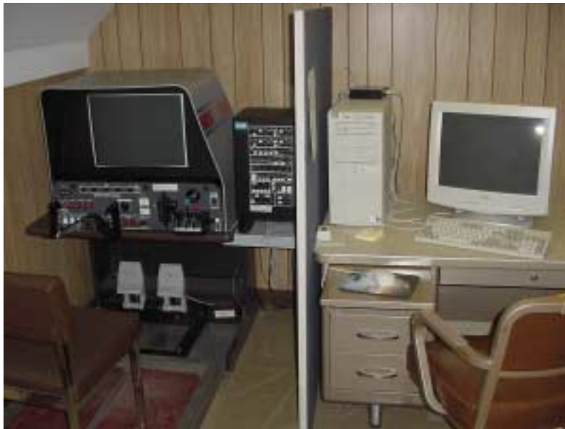
Figure 1. PCATD from Aviation Teachware Technologies (ELITE) v 6.0.2, and flight controls by Precision Flight Controls.
